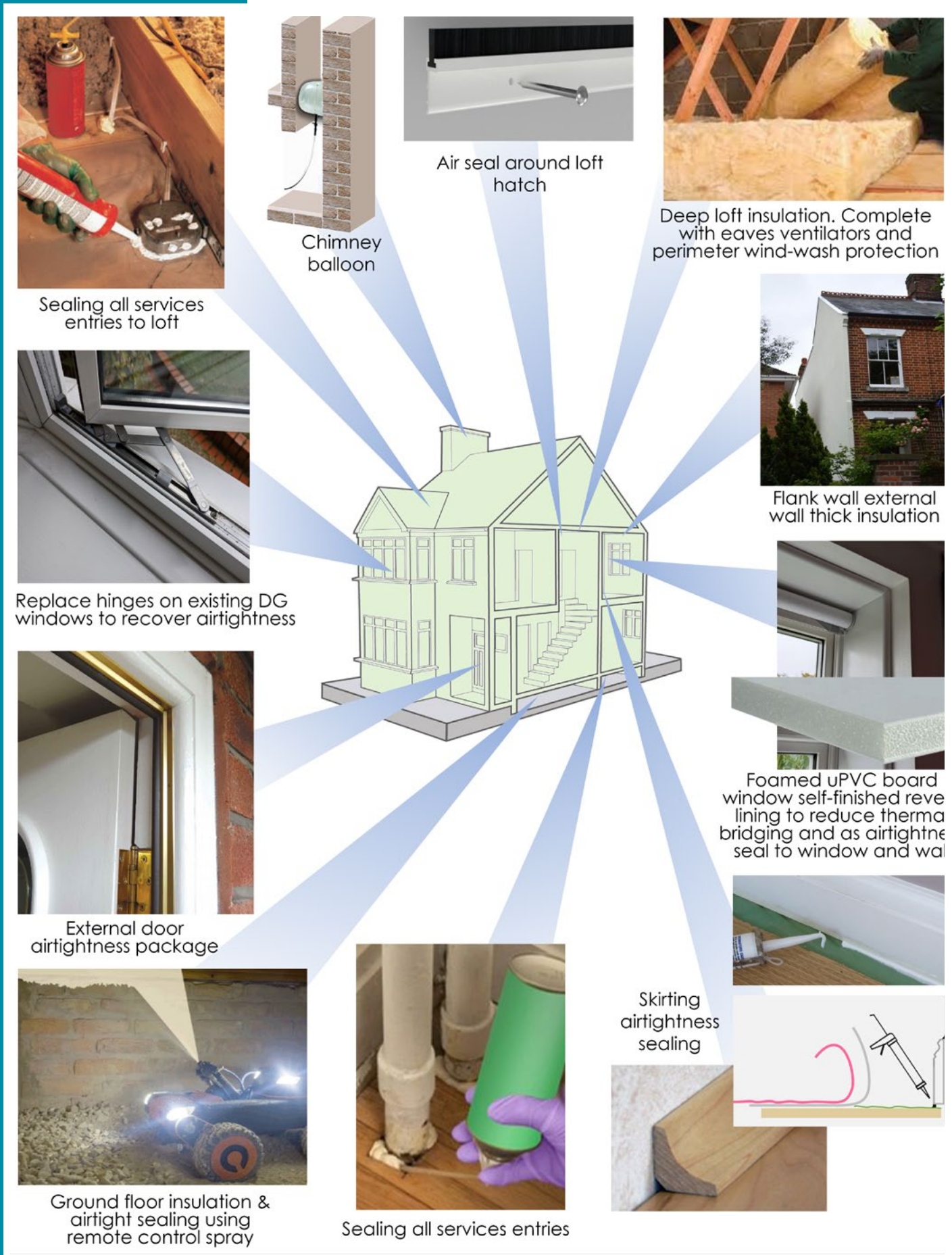
Figure 4.3 Typical fabric measures found to be sufficient for airtightness, thermal bridging, and thermal insulation for the illustrative example to meet the BASIC energy target.
