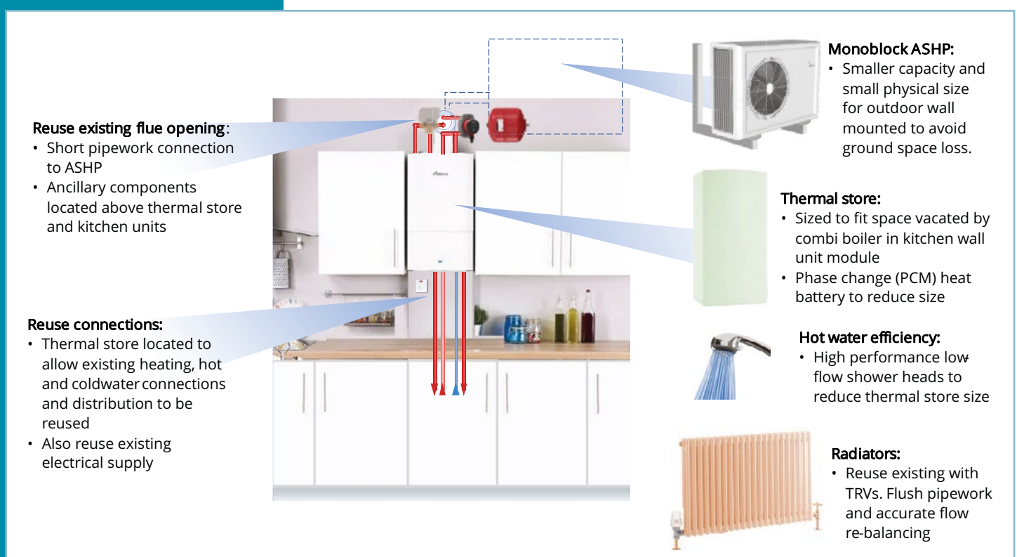
Figure 4.11 Simplified heat pump switch over installation
