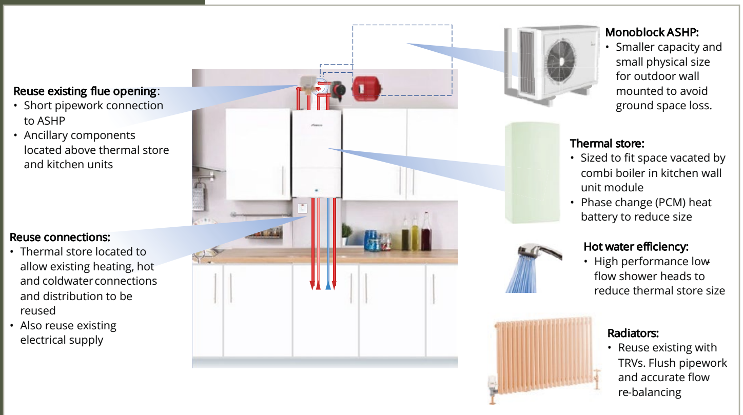
Figure C.8 – Simplified heat pump switchover installation.
